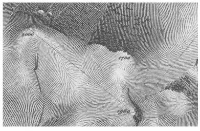
b) Terrain rendering using slope hachuring (Lehmann, 1843)
