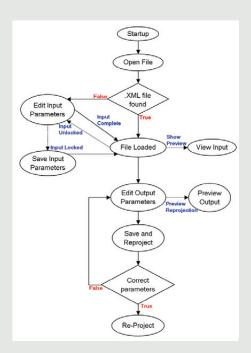
Figure 16. Diagram of reprojection flow
