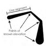
Figure 5. Showing the location of points of known elevation and line width changes in between.
