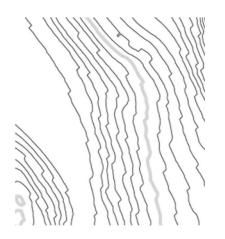
*Figure 7. Jagged contour lines resulting from corduroy effect on DEM data.*
